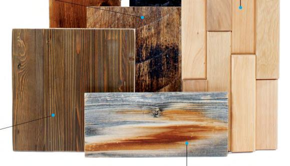
Kirei harvested Douglas fir and hemlock fir from demolished buildings in the Pacific Northwest to create its Windfall reclaimed-wood engineered panels. Made from 5/s", 3/4", and 1" wood strips laminated together, the 3/4"-thick interior wall panels come in 27"-by-96" and 48"-by-96" sizes. The wood may be unfinished, finished in a clear coat, or stained and prefinished in anthracite (shown), mocha, ivory, and leather. • kireiusa.com • Circle 105
