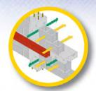
Channel flow: Air flowing through channels, cracks, or joints in the building envelope.
