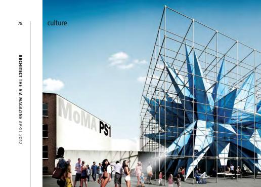
Wendy's skin features nylon fabric treated with titaniumoxide nanoparticles that neutralize airborne pollutants.
