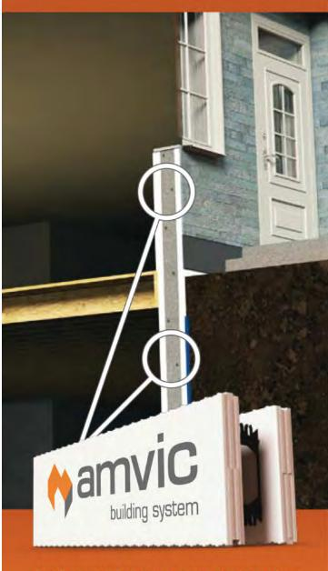
Our Expanded Polystyrene forms stack together and interlock; simply add rebar, brace, and pour. With the concrete set, forms remain as insulation, which can then be finished to suit your design.
