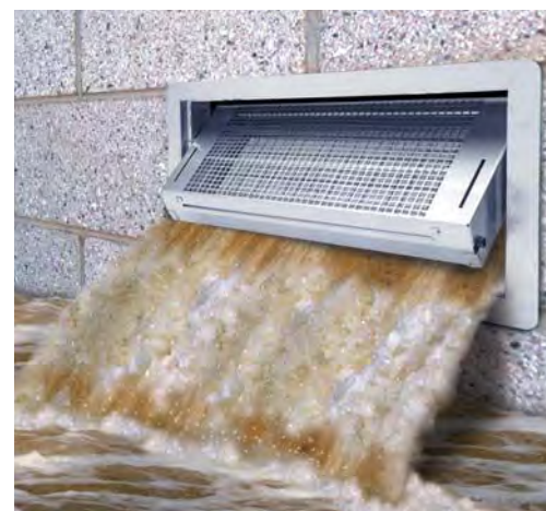
Flood vents provide wet floodproofing, automatically equalizing the hydrostatic pressure acting upon the structure. Photo by Smart Vent Products, Inc.
