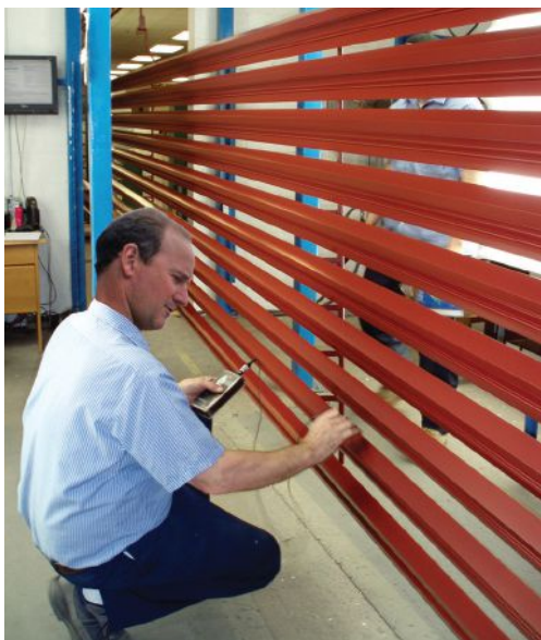
Unlike quality control of anodized coatings, which is very manual, there are electronic tools that can be used for quality checks on painted surfaces.
