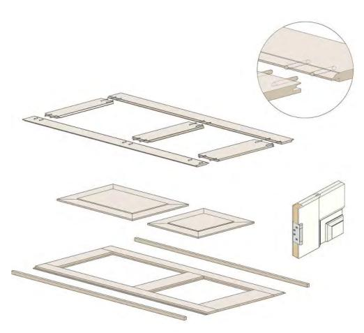
In the continuous lamination method the stiles and rails of each half are joined using a cope and stick method, and a wood edge channel is grooved into the face of each half door to accept the wood edge.
