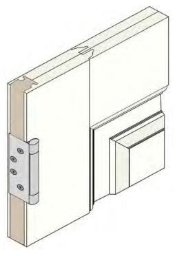
Keyed-in poplar wood edges run the full length of the stiles, and add stability, durability, and screw holding strength.
