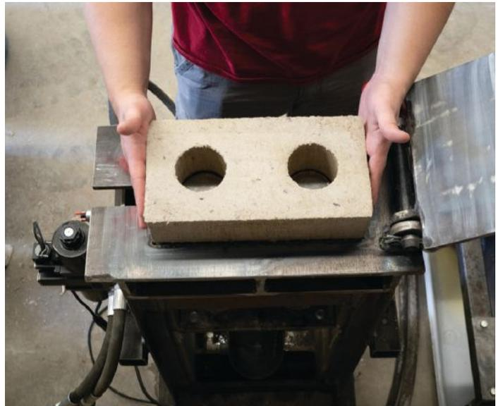
The pressing process for a drywall waste block can occur on-site using portable machines or off-site using existing machinery at conventional CMU plants.
