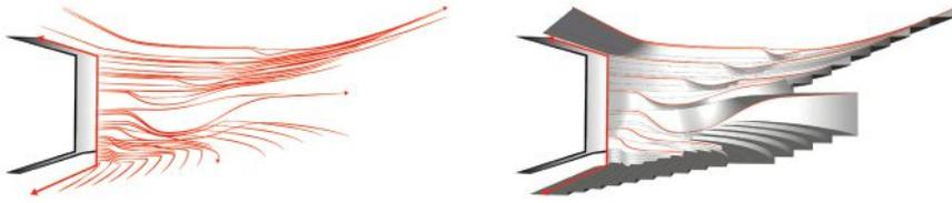
Fabricating the steam-bent oak panels required a combination of traditional craftsmanship with laser scanning and projection. The augmented reality construction process placed Trahan Architects' scripted layouts into the real world, ensuring the accuracy of the millwork's form and placement.
