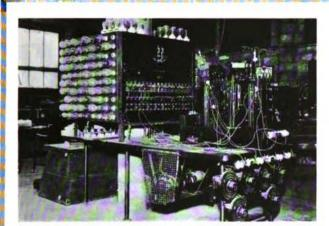
Switch and Socket Testing Machine
