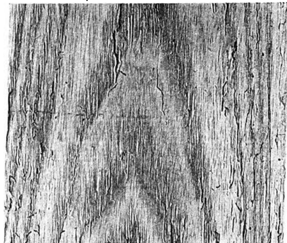
Damage to hardwood by Lyctus powder-post beetles (Fig. 2)
