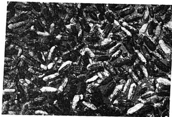
Pellets of finely digested, excreted wood expelled by powder-post beetle vrilletta sp. These droppings are a warning that woodwork is infested.
