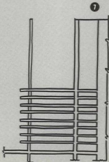
**Telecomputing Facilities, Chatsworth, California:** T. Y. Lin & Associates, structural engineers. Upward prestressing balances weight of 120-foot precast T-beams which frame the building. Additional prestressing was applied to balance weight of in-place post-tensioned concrete roof slabs. Roof deck is a parking area without membrane.
