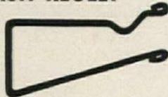
SA or SF. Placed in concrete for metal sash, sliding doors, etc. Requires no grouting or caulking.
