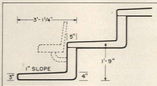
Prestressed angle slabs used as seat decks have a 1" slope for proper drainage.
