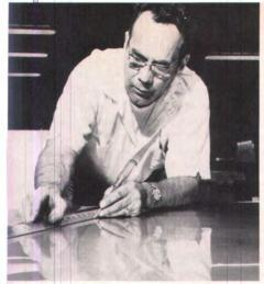
The stainless sheets marked up here for press vork, were formed by the mechanical conractor, Temp-Control Corp., Portland.
