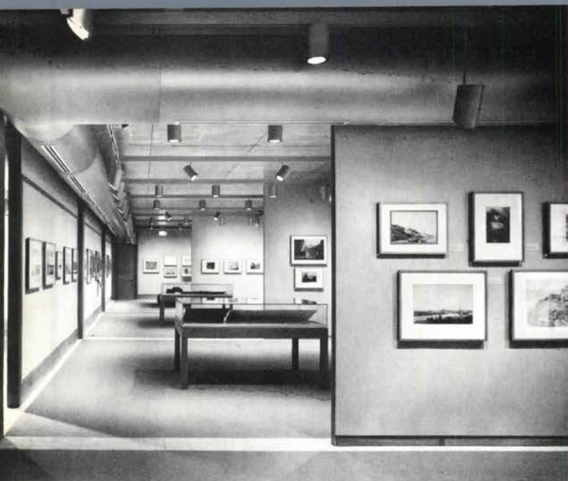
The fourth floor study gallery (right) is divided into 20-foot bays, each with its own skylight. Running through the second floor exhibition galleries (above) are large, cylindrical stainless steel airconditioning ducts.
