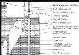
Wing walls of Acme Brick intersect the main form and carry the implied wall mass above. In addition they provide solar shading.
