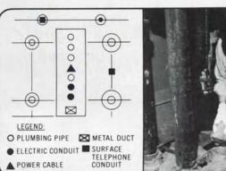
was used to seal openings of various sizes. These openings provided access for steel pipe, copper pipe, steel conduit, metal air ducts and power transmission cables run through a fire-rated floor.
