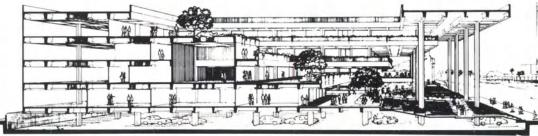
Four above-grade office and courtroom levels, photo and section at left, are stepped back to provide the open terraces that largely supplant interior corridors. The stepping also creates a major multilevel plaza at the heart of the building. Despite this internal complexity, a powerful building cornice built right to the property line, below, defines a simple overall building form and establishes a new standard for urbane downtown planning in the community.
