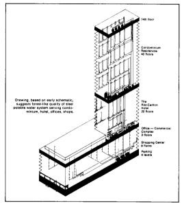
When the time came to specify the pipe for the potable water system, project planners scanned competing materials and agreed it had to be steel.
