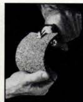
Bending at 0°F for Cold Flex: No Failure.
