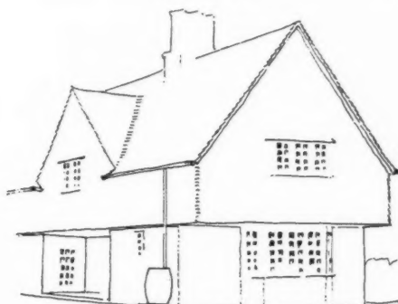
FIG 3 LIGHT WEATHER TILED WALLS OVERHANG BASE.
