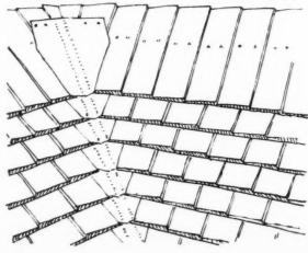
The ridge of the roof may be covered with a pair of grooved and rebated oak saddle boards set together at right angles. The saddle boards are made in long lengths and where end to end joins are necessary a dovetail lap joint should be made (see Fig. 1).
