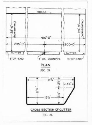
and the cross section of the gutter is approximately as shown in Fig. 21.
