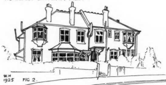
HOUSES AS DESIGNED TO COMPLY WITH THE BY-LAW RELATING TO THE PARAPET ON A PARTY WALL.
