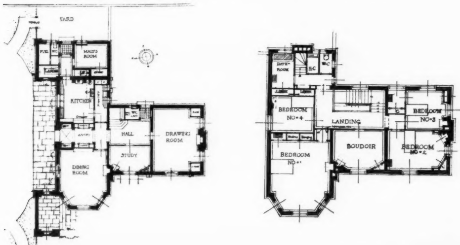
A house at Leamington (1923). The entrance front, and, below, plans of the ground and first floors. This house was planned to make use of an existing garden to the south-west. On the second floor are four bedrooms.
