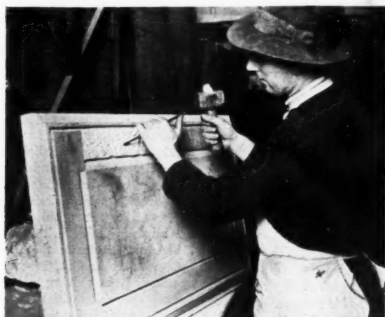
Left, figure three. Cutting an ornamental border upon a slab. The channels on the lower part of the slab show how the depth of background for the ornament is first settled. A chisel with the blade ground round at the corners is used to form the rounded hollows in the leaves. The chisel has a cup-shaped hollow in its driving end, whose edge bites into the soft iron head of the hammer. Right, figure four. Cutting an ornamental boss in a block of Portland stone with mallet-headed chisel and beechwood mallet. To support the block during the operation it is bedded against two heavier blocks with plaster of Paris.
