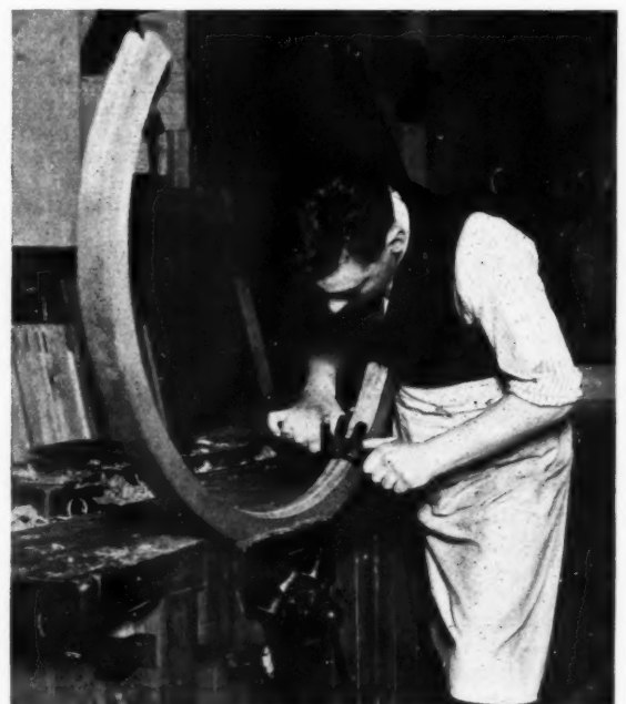
Left, figure five. Using the shoulder plane. An extremely sharp iron and a very fine set are needed in removing a thin uniform shaving from the end grain of the wood to assist the other shoulder to come up in contact with the style. It is the ambition of the good joiner to produce good shoulders without the use of the plane. Right, figure six. "Sticking" an ovolo mould on a circular head on the solid by hand with an iron spokeshave. The direction of the grain of the wood has to be considered, and the joiner faces the other way in moulding the part projecting to the left of the vice.
