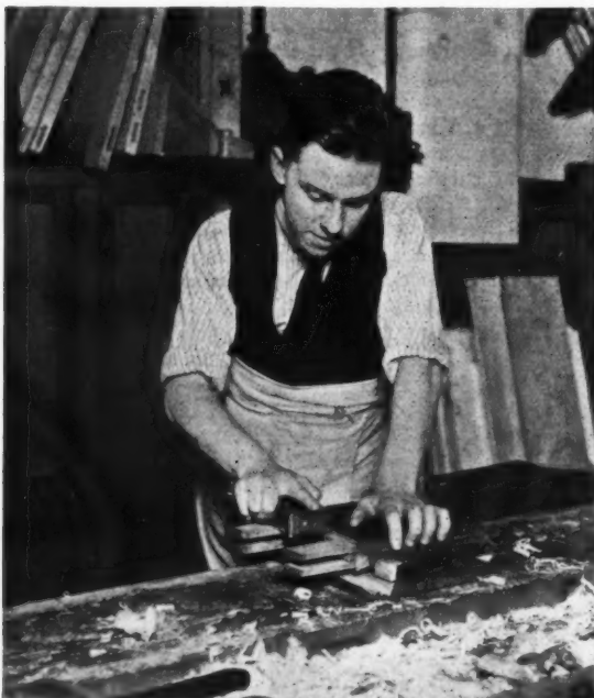
Left, figure five. Using the shoulder plane. An extremely sharp iron and a very fine set are needed in removing a thin uniform shaving from the end grain of the wood to assist the other shoulder to come up in contact with the style. It is the ambition of the good joiner to produce good shoulders without the use of the plane. Right, figure six. "Sticking" an ovolo mould on a circular head on the solid by hand with an iron spokeshave. The direction of the grain of the wood has to be considered, and the joiner faces the other way in moulding the part projecting to the left of the vice.
