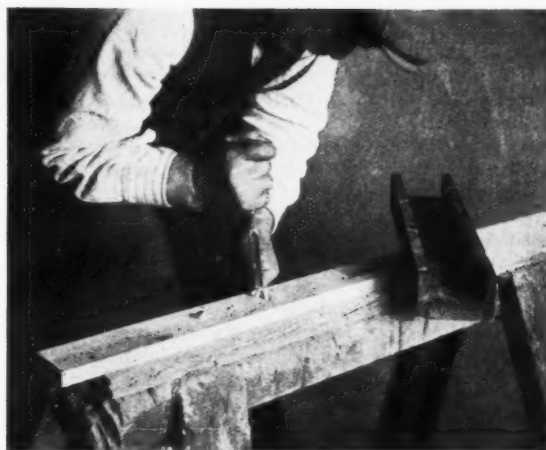
Figure five, left. Cutting a mitre in the mitre-box. The two saw-kerfs in the sides of the box are set out at angles of 45 deg. to the line of its length and guide the saw blade as it is used to cut at a similar angle across any moulding placed in the box. Figure six, right. Scribing a piece of ovolo moulding to surround a window frame. The end of the moulding has been cut to a mitre in the mitre-box to provide an accurate setting out line for the gouge to cut to.
