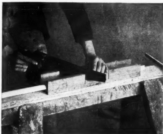
Figure five, left. Cutting a mitre in the mitre-box. The two saw-kerfs in the sides of the box are set out at angles of 45 deg. to the line of its length and guide the saw blade as it is used to cut at a similar angle across any moulding placed in the box. Figure six, right. Scribing a piece of ovolo moulding to surround a window frame. The end of the moulding has been cut to a mitre in the mitre-box to provide an accurate setting out line for the gouge to cut to.
