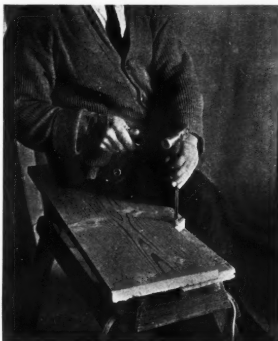
Figure four. Cutting a hollow corner with the help of a gouge. A straight cut has been made with a saw, and the curve is being chipped to shape. In the machine shop such work would be performed with the band saw.
