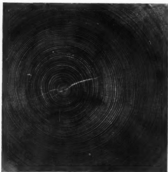
Cross section of Pitch Pine, showing slight shakes along medullary rays.
