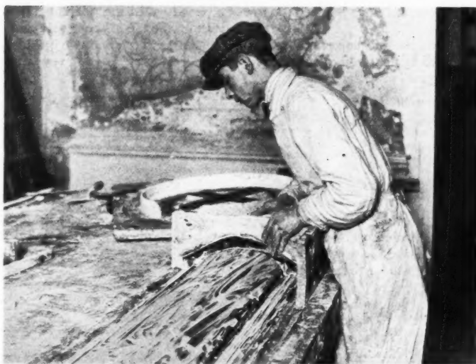
Figure four. Trying the reverse profile mould in position while the core of the reverse mould is being built up with old casts and a thin layer of new plaster.
