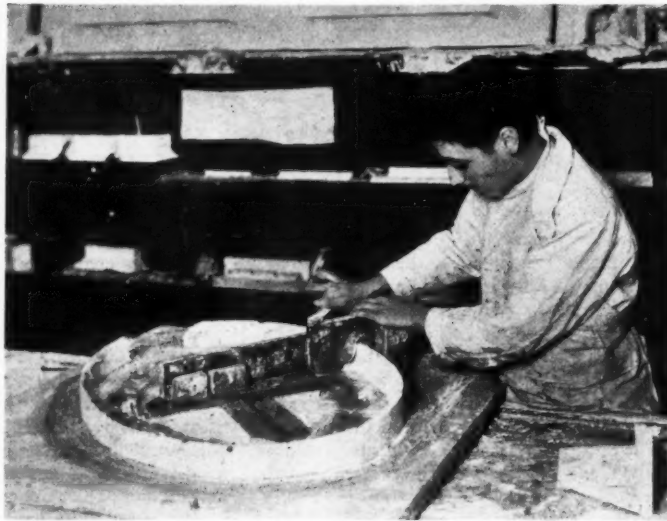
Figure two. Trying the effect of the "profile mould" and "trammel" on the elliptical or, so-called, "oval" medallion. The raised margin of the ellipse is formed with canvas and plaster on a basis of long nails driven into the plaster-faced "moulding-board."
