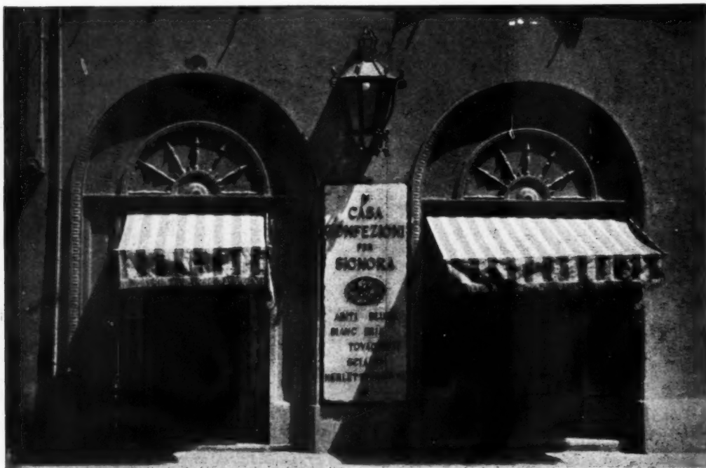
The modiste shop of Messrs. Delli and Botti, Via Sistina, Rome. By Professor Venturoli. The duality of these arched openings is resolved by means of a generous rectangular sign made out of a single block of travertine. On this block brass letters are applied. The wall is finished in stucco painted buff.
