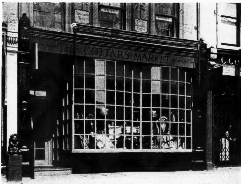
The Cottars' Market, Brompton Road. By Decimus. This is a type of intimate shop where the use of a small Georgian pane is appropriate and well justified. The effect of the glass set at different angles gives an unusually interesting light reflection. The lettering in the fascia is refined and distinctive, but the connection between this and the window is not of the happiest. In the old days the fascia would have followed the line of the shop front (as in the famous double-bowed front in Dorking High Street). The complete "frame" to the picture is missing, owing to the retention of the existing pilasters and consoles, which are out of character with the new front.
