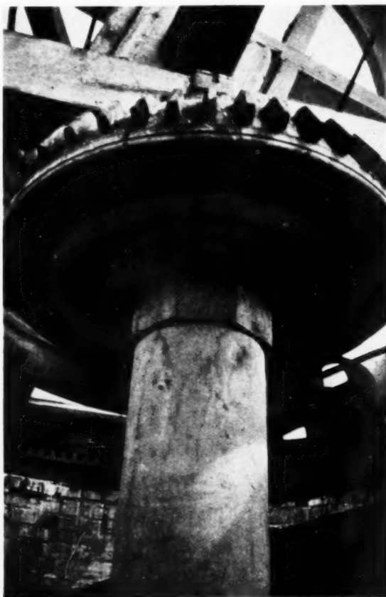
Ringstead Mill, near Hunstanton, Norfolk. Converted by H. C. Hughes. The great oak machinery is retained. It is extremely decorative and takes up little room. The illustration shows the wallower at the top of the main shaft of the mill.
