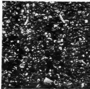
A section of concrete made with grey cement and shingle in the proportion of four to one, and treated with Redalon liquid, which enables the cement skin to be brushed off after the centering has been removed.
