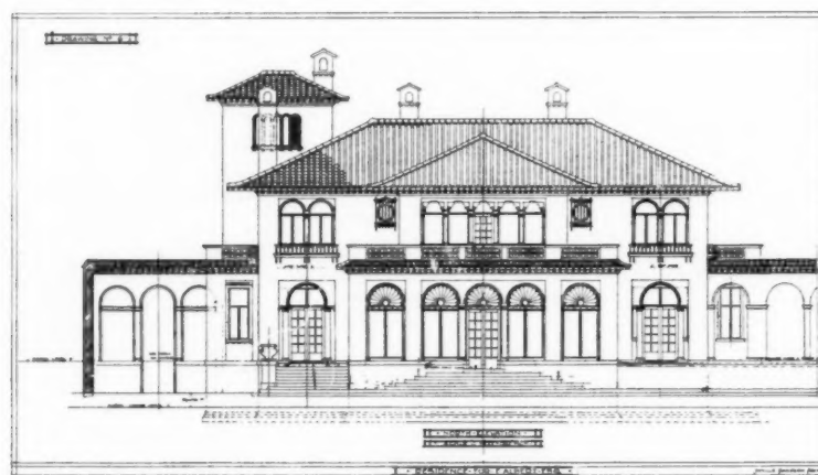
House in Sydney. By Neville Hampson. Elevations. The roof is covered with half-round tiles of various brilliant colours, and the walls are plastered and finished a cream pink. The casement windows are of brass, turned green. The eaves of the roof project 4 ft. and the under spars are painted a deep purple.
