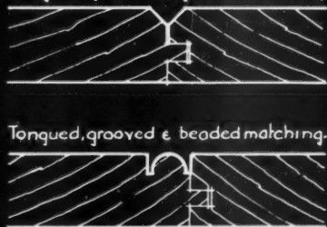
TYPES OF JOINTING TO MATCHING: Tongued, grooved, & V. jointed matching.
