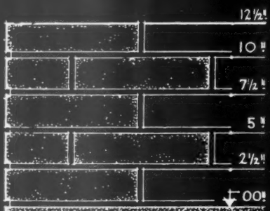
2" BRICK WITH \frac{1}{2}'' JOINTS:
