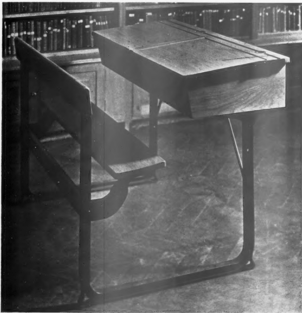
A standard type of two-seater school desk with a flush top, locker, and I-section side members for stiffness. [Educational Supply Association.]
