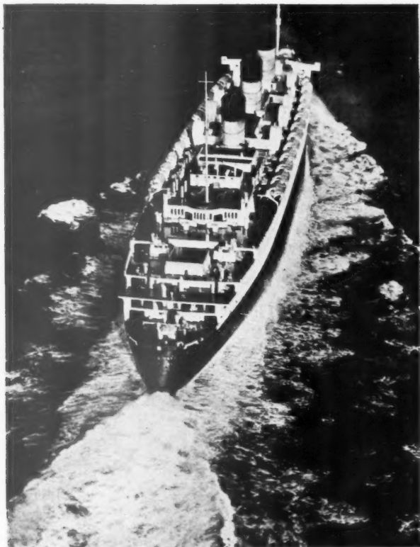
British and French. Two photographs which show interesting differences in the naval architecture of the two fastest liners. The utilitarian placing of the deck gear and superstructures of the "Queen Mary" (left) contrast with the emphasis on clear deck space which is the striking characteristic of the "Normandie" (right).
