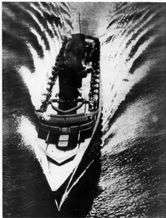
British and French. Two photographs which show interesting differences in the naval architecture of the two fastest liners. The utilitarian placing of the deck gear and superstructures of the "Queen Mary" (left) contrast with the emphasis on clear deck space which is the striking characteristic of the "Normandie" (right).
