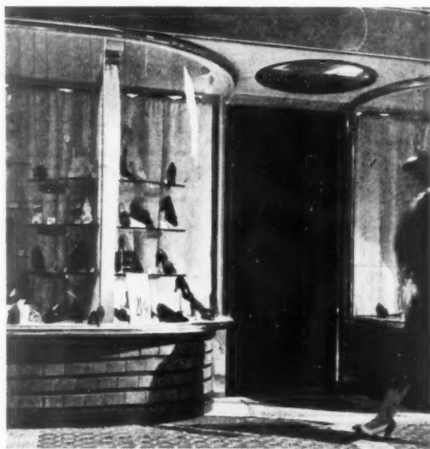
Doorway to the London Shoe Company's shop in Regent Street. Stallboard is of glazed brick and the window framing in brass. The curved windows flanking the entrance are expensive, but tempt the passer-by to enter.
