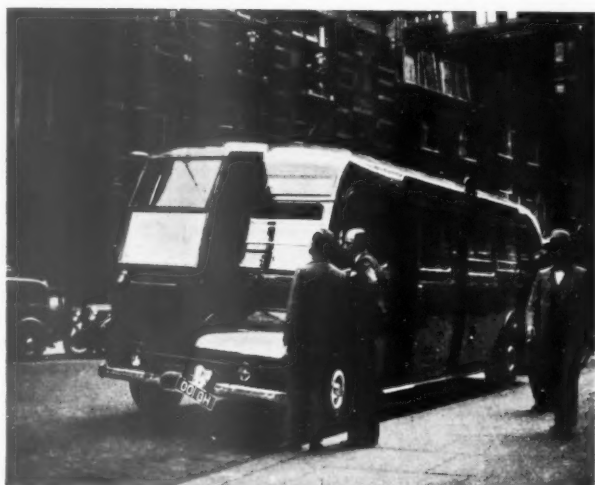
An experimental Green Line bus photographed while being inspected at 55 Broadway. To the casual observer the principal features of the bus were the high seat of the driver, external sliding doors, fast acceleration and a very wide lock.
