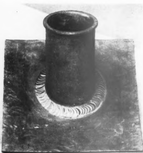
A typical leadburned detail made up from flat sheet.
