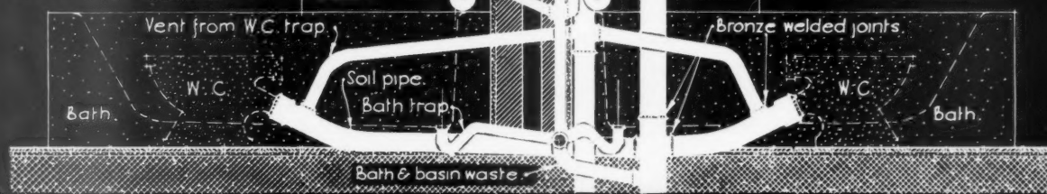
ELEVATION OF PLUMBING IN COPPER PIPING TO TWO ADJACENT BATHROOMS.
