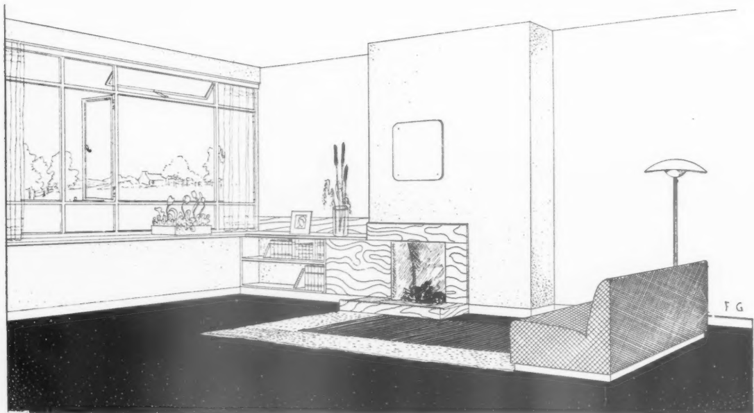
Typical interior showing 9-in. side wall under full width of window with lintols dropped from floor above and an infilling panel under.
