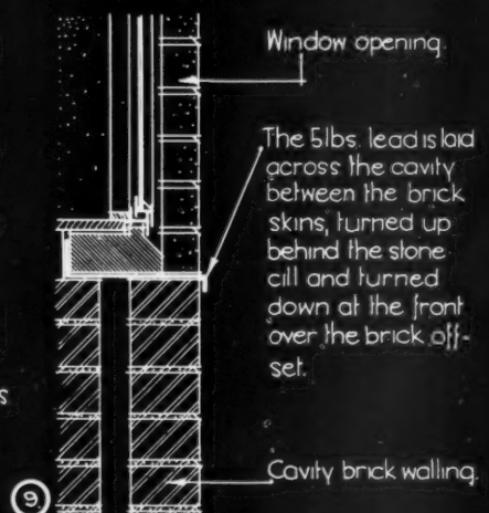
WEATHERING TO A BRICK-ON-EDGE OFFSET BELOW A STONE CILL.
