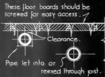
Section showing alternative fixing for pipes running at right angles to joists.
