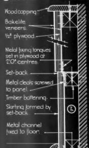
Wall coverings in 1/2! plywood are veneered on both sides with Bakelite sheet. Backing veneer prevents absorption of moisture and sogging which occurs when plywood is veneered on one side only.
