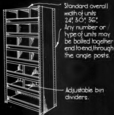
DIAGRAM 3: Closed type shelving with all shelves fitted with bin fronts & the upper ones with bin dividers.
