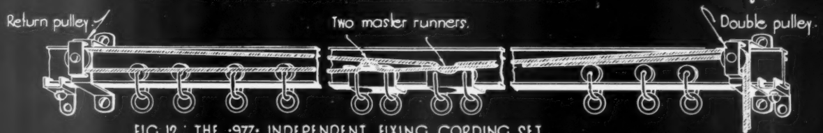
FIG. 12 : THE '977' INDEPENDENT FIXING CORDING SET.
