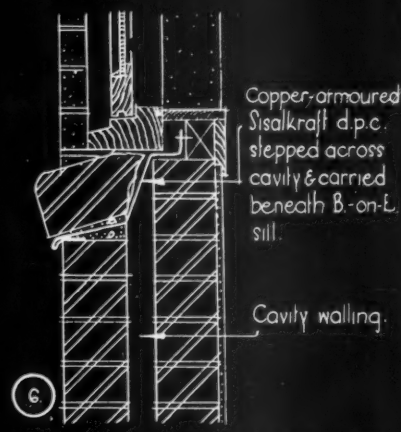
6. WATERPROOFING BOTTOMS OF OPENINGS.
