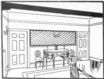
The photograph above illustrates a typical installation of Invisible Radiant Panels. The sketch on the left shows the location of the panels.
