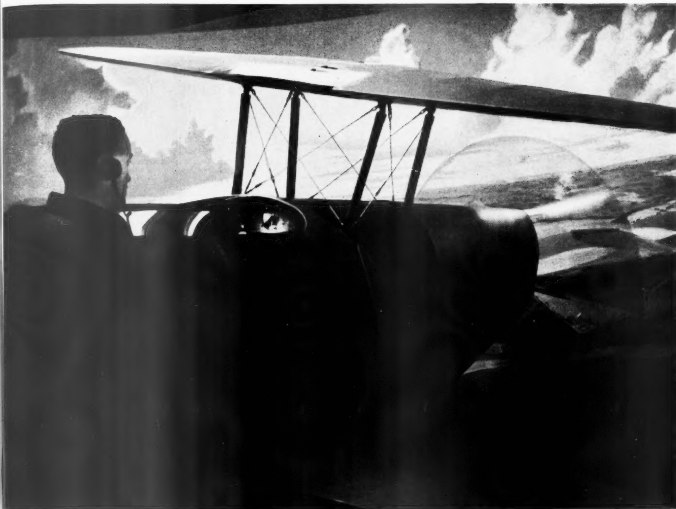
7—The Link Trainer banking. The cellulose film propeller gives right obscurity ahead and the upper wing the right limitation of vision for a primary trainer.
