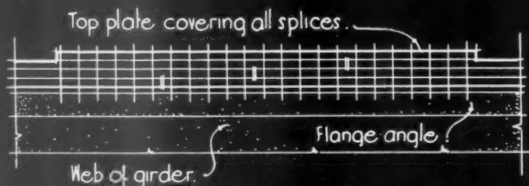
FIGURE 2A: STAGGERED SHOP SPLICES FOR SEVERAL FLANGE PLATES.
