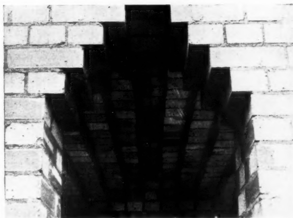
4—Test of brick shelter, with brick corbel roof, to seat eight persons. 5 and 6 show that the corbel roof was not damaged externally or internally.
