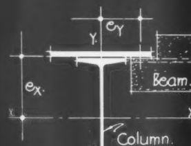
FIGURE 3: Y-axis eccentricity due to joist-flange connection.
