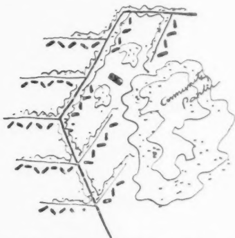
B: This, showing the principle on which one of the prize-winning layouts is based, is an attempt at giving an indeterminate appearance from the air by using a zig-zag pattern of roads and, in contrast to scheme A, a pepper-and-salt arrangement of houses. The road system could not be easily worked into the normal rural pattern, and it is doubtful if a pattern based on regular irregularity is likely to be less obvious from the air than a simpler rectangular one.
