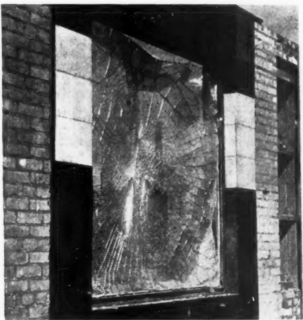
After second test (2-lb. bomb at 20 ft.) of 1/2-in. plate glass window protected on back with netting firmly glued to glass. A typical example of the "diaphragm" fracture which occurs when blast hits glass at right angles. After first test, glass bulged forward 2 to 3 ins. After this second test, glass came to rest with backward bulge of 3 to 4 ins. at centre.
