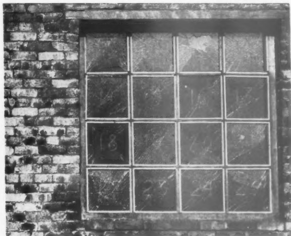
A frame of 15 panes of wired glass and one of 1/2-in. rough cast, double rolled, after the final test at distance of 10 ft. approximately equivalent to 500-lb. bomb at 50 yds. All the wired glasses, though badly cracked, have held. The rough cast pane had fragments dislodged.
