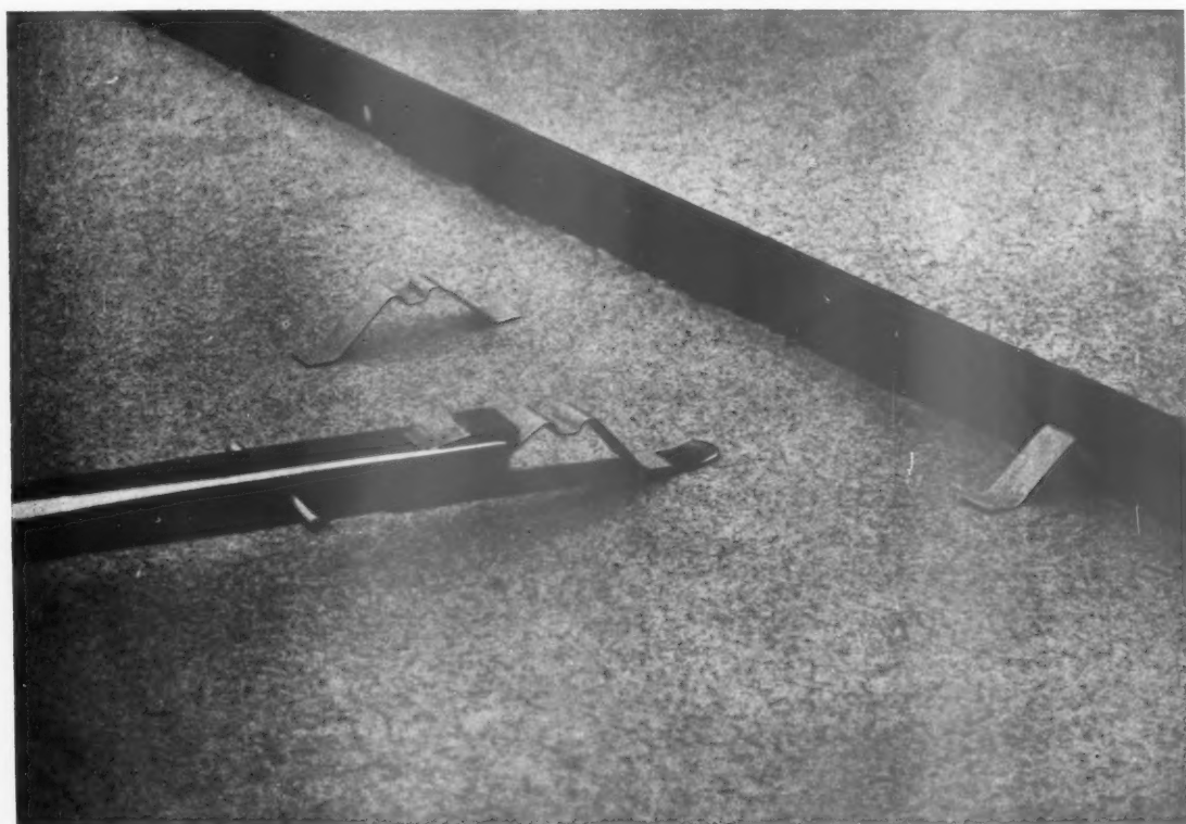
Close-up photograph of special tool for insertion of spring clips through the slots in the back of metal cover strips.
