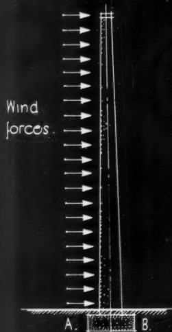
FIGURE 3: EXPOSED STACKS, SPIRES, WATER TOWERS, ETC. The wind forces may cause an uplift at point A, in which case the foundation at B must be heavy enough to counteract this tendency.
